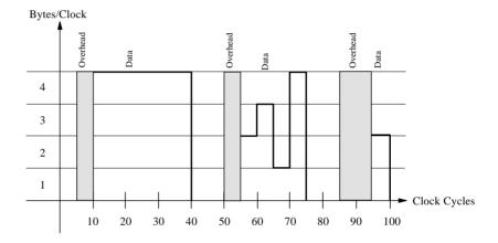
In the diagram above, the clock cycles are indicated horizontally. The vertical axis represents the **address/data** bits. In 32-bit systems a maximum of four bytes can be transferred per clock cycle. The actual number of transferred bytes is determined by the **byte enable** bits.
