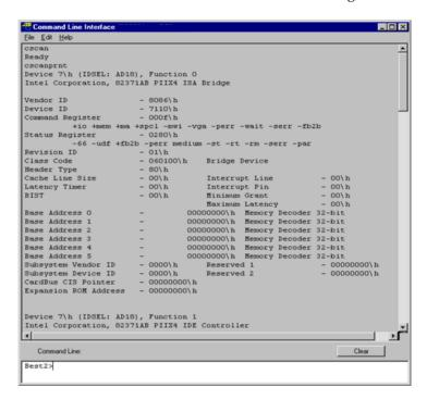
NOTE The Command Line Interface only works with a proper data connection to an Agilent Exerciser and Analyzer testcard plugged into the system under test.
