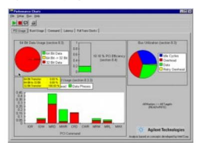
This window presents the performance of your system under test on five different tabs. The *PCI Usage* tab (as shown above) presents general traffic statistics like the bus utilization and the PCI command usage.
