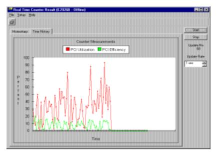
NOTE In offline/demo mode, running the real-time measurements does not cause an error message but produces random values to be displayed.
